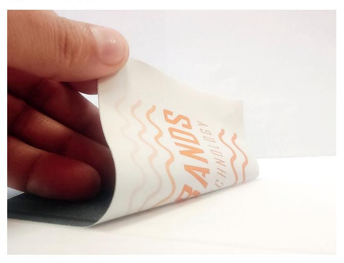
E-print® technology consists on printing electronic circuits using high-end Heat-Transfers technology.
